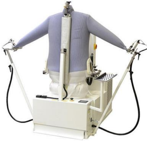
Figure.5.4 Foam finishing machine
